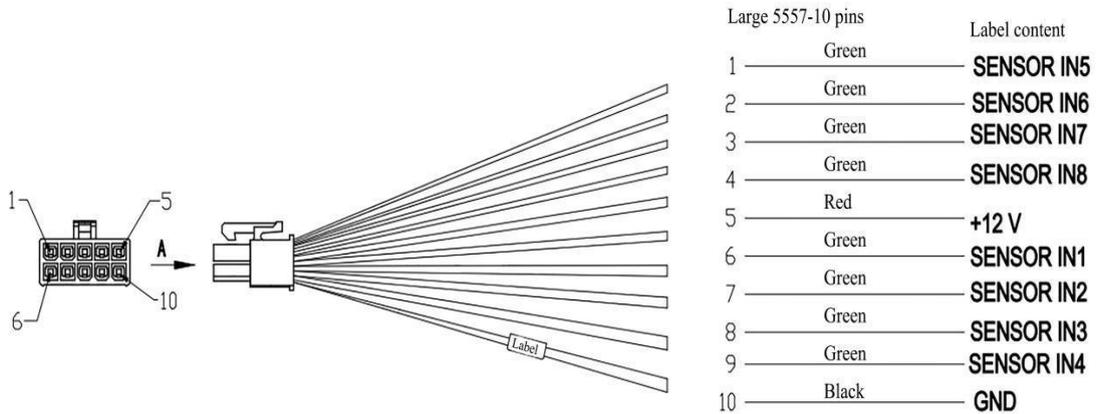
Speed detection cable connector pinouts:
