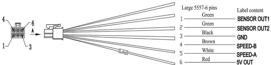
CAN signal cable connector pinouts:
