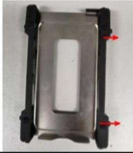
Take out the hard disk damper assembly and open one of the dampers to a certain angle (Note: If the hard disk is 9 mm thick, tear off the two rubber pads in the bracket; if the hard disk is 7 mm, keep the rubber pads, as shown in the figure above)
