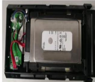
Connect the SATA cable to the hard disk, and install the hard disk assembly into the hard disk cartridge, as shown in the figure above
