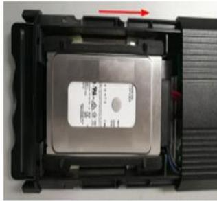
Loosen the 4 screws at the bottom of the hard disk cartridge with a Phillips screwdriver, and pull out the upper cover of the hard disk cartridge, as shown in the figure above
