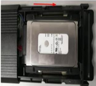
Install the upper cover and tighten the 4 screws at the bottom of the hard disk cartridge, as shown in the figure above
