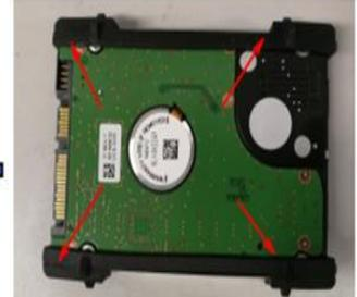
Hold the dampers at the correct location and press the four corners of the two dampers with hands to make them stick to the bracket, as shown in the figure above
