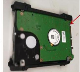
Insert the hard disk cartridge obliquely into one side
